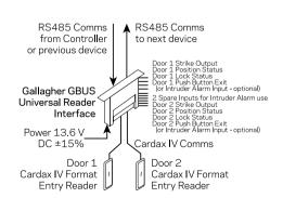
Two Cardax IV format entry readers (with push button exits) connected to the Gallagher GBUS Universal Reader Interface for the access control of two doors.
