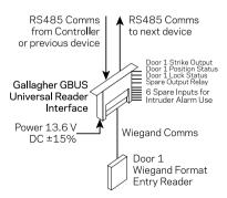
One Wiegand format reader connected to the Gallagher GBUS Universal Reader Interface for the access control of one door.
