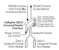
Cardax IV format entry and exit readers connected to the Gallagher GBUS Universal Reader Interface for the access control of one door.
